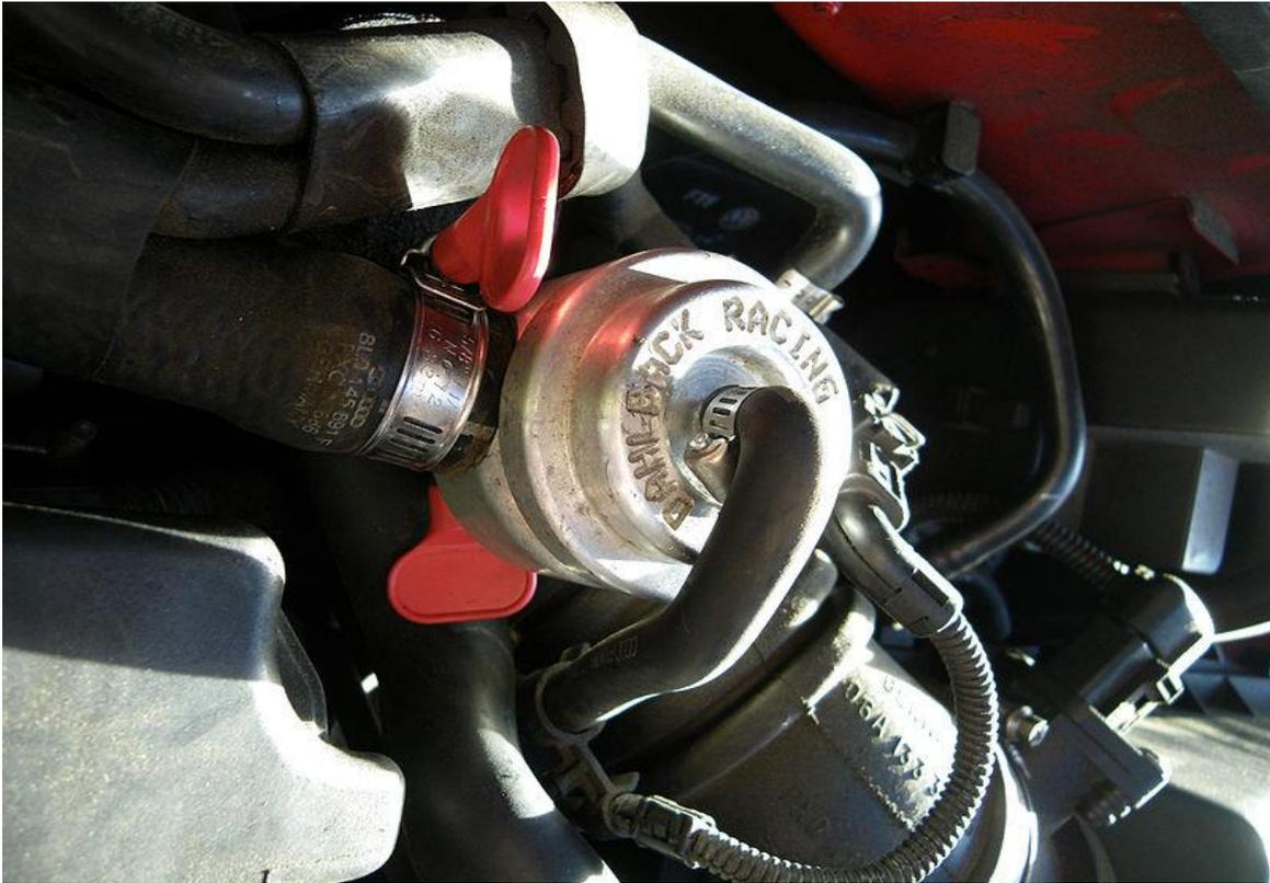
**Fig 1.10A recirculating type anti-surge valve**
