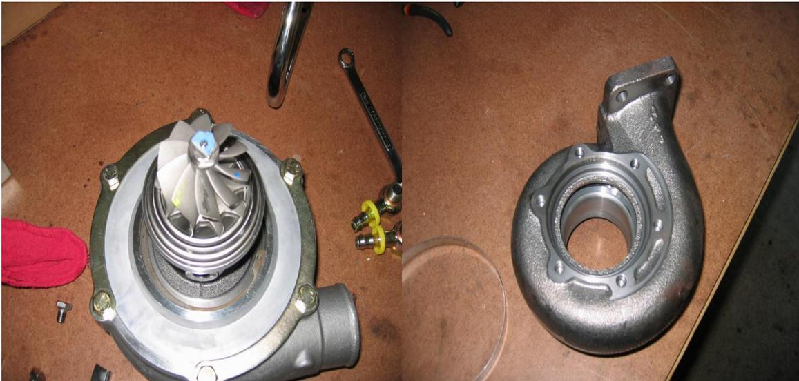
**Fig 1.4 Turbine side housing removed.**
