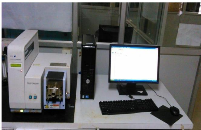
**Fig 4.5 Thermo gravimetric analyzer**
