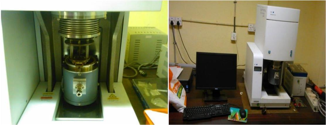
**Fig 4.9 Dynamic mechanical analyzer**
